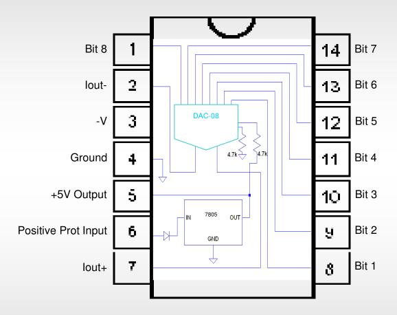
+5V voltage regulator and DAC08 D to A converter, residing in a single package. The +5V regulator input is protected by a series diode.
